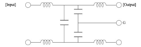
Figure 4.12 AC noise filter (recommended)
